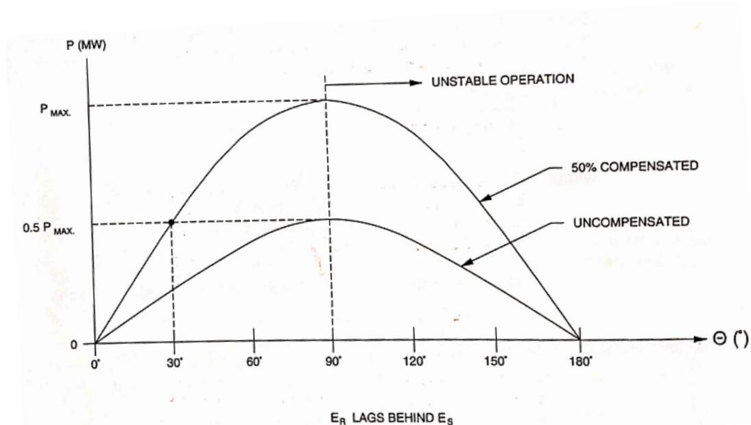
**Fig 17.3** Power transfer capability of a transmission line with and without series compensation.
