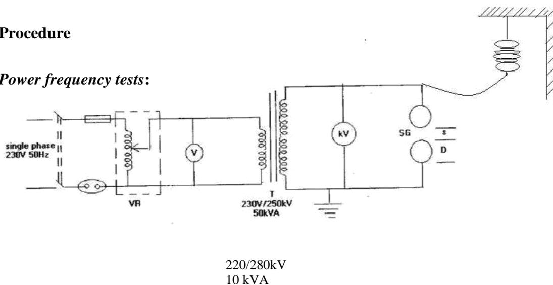
**Figure 6.1:** Circuit Diagram
