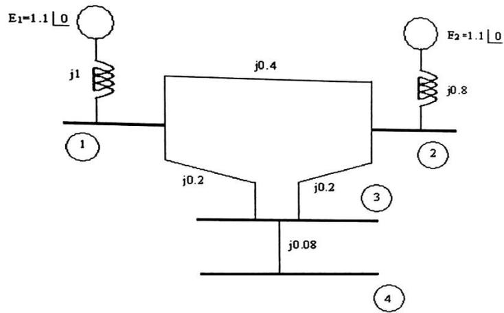
Fig 2.1 Single Line Diagram
