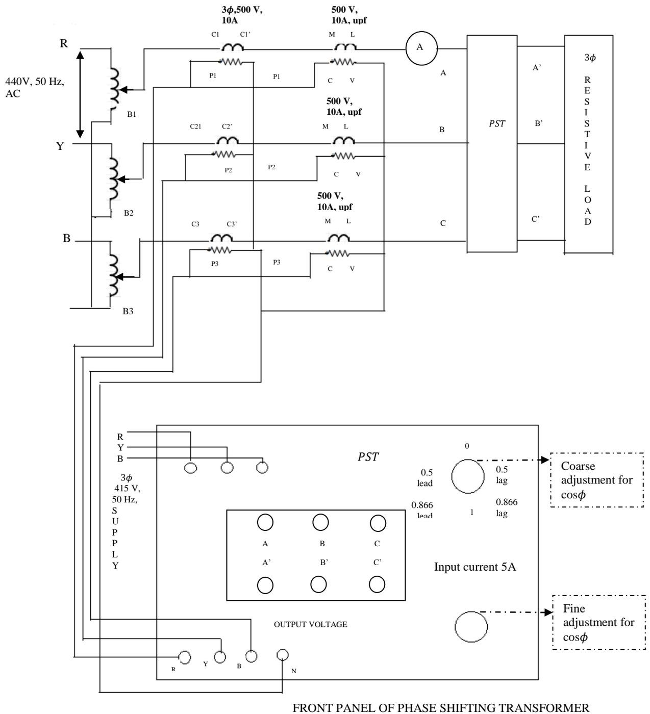
**Fig 15.1:** Connection of three phase energy meter and phase shifting transformer.
