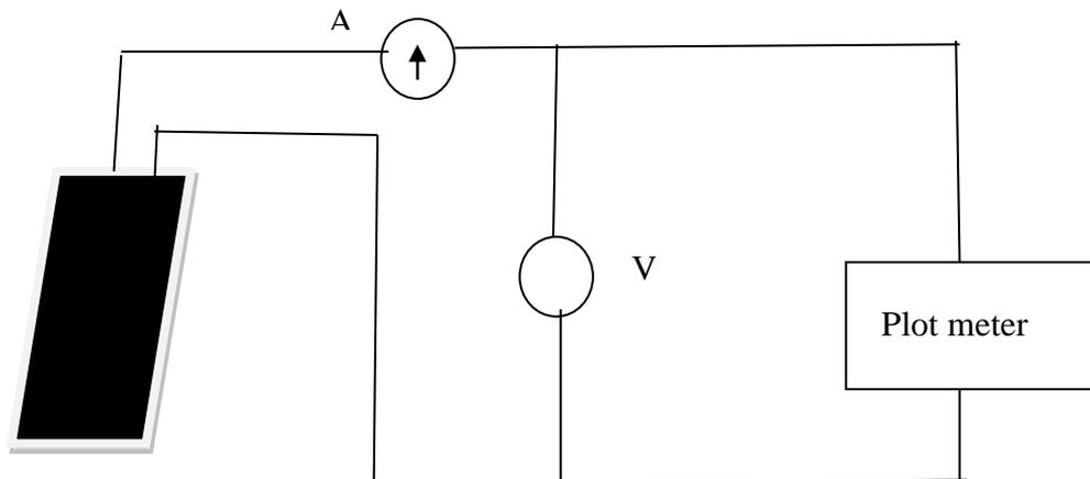
**Fig 14.3:** Circuit diagram for P-V characteristics
