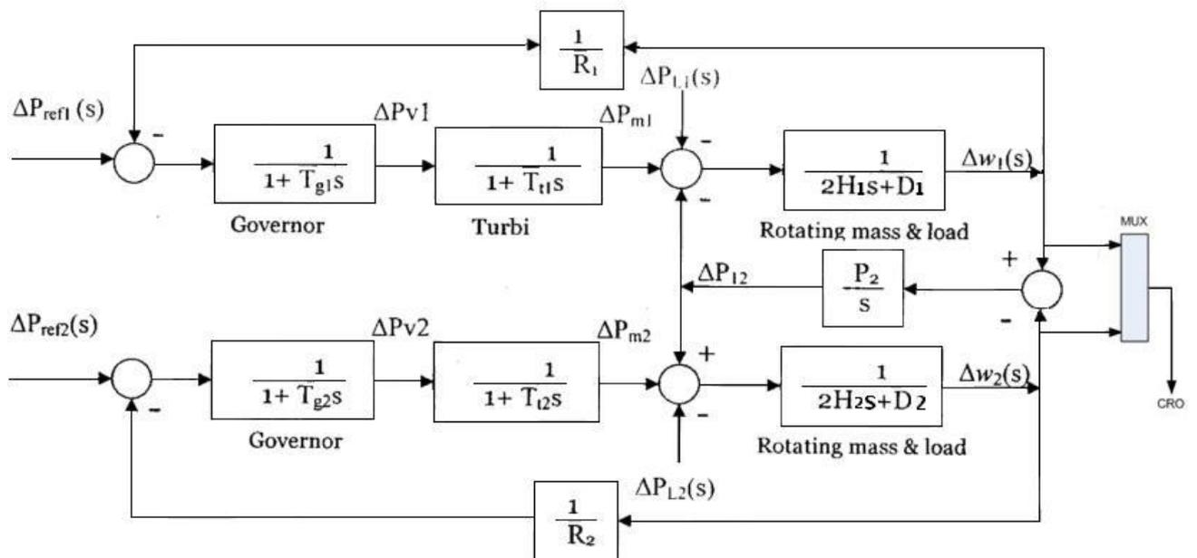
**Fig 5.2:** Two area system with only primary LFC Loop
