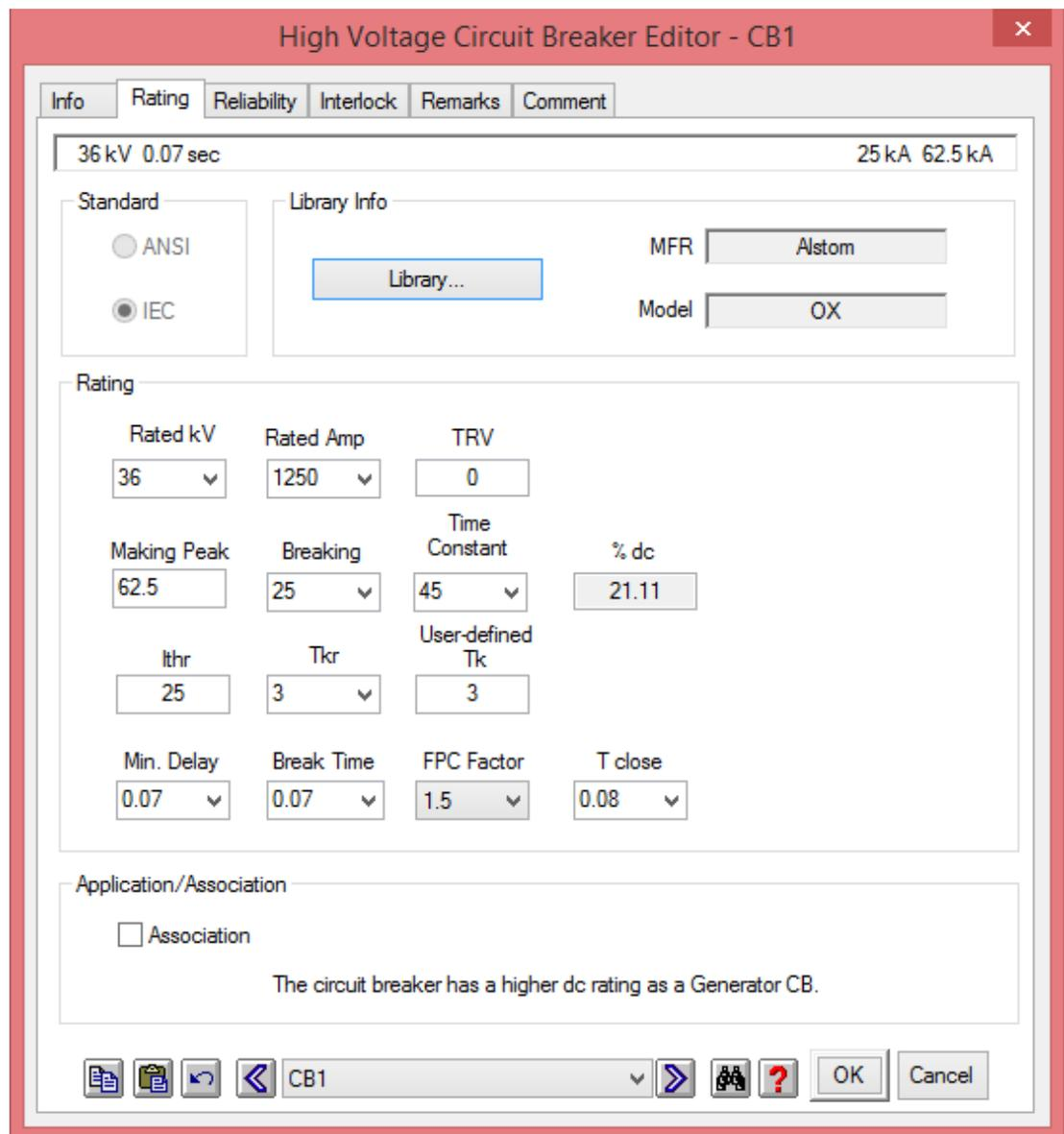
**Fig 16.4:** High Voltage Circuit Breaker Editor
