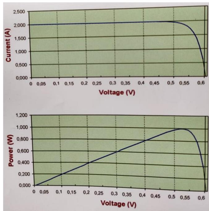
**Fig 14.1:** Characteristic curves of Solar PV module
