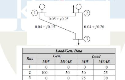
2. Considering Bus 1 as slack bus, use DC load flow to obtain one iteration of load flow solution for the system shown below. (K2, K3)(PO1,PO2,PO3,PO5)
