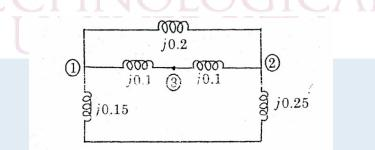
12. For the reactance network shown in figure find Z bus by direct determination (14)
