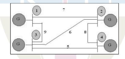
2. For the network in Fig, form the primitive matrices [z] & [y] and obtain the bus admittance matrix by singular transformation. (K2, K3)(PO1,PO2,PO3,PO5)
